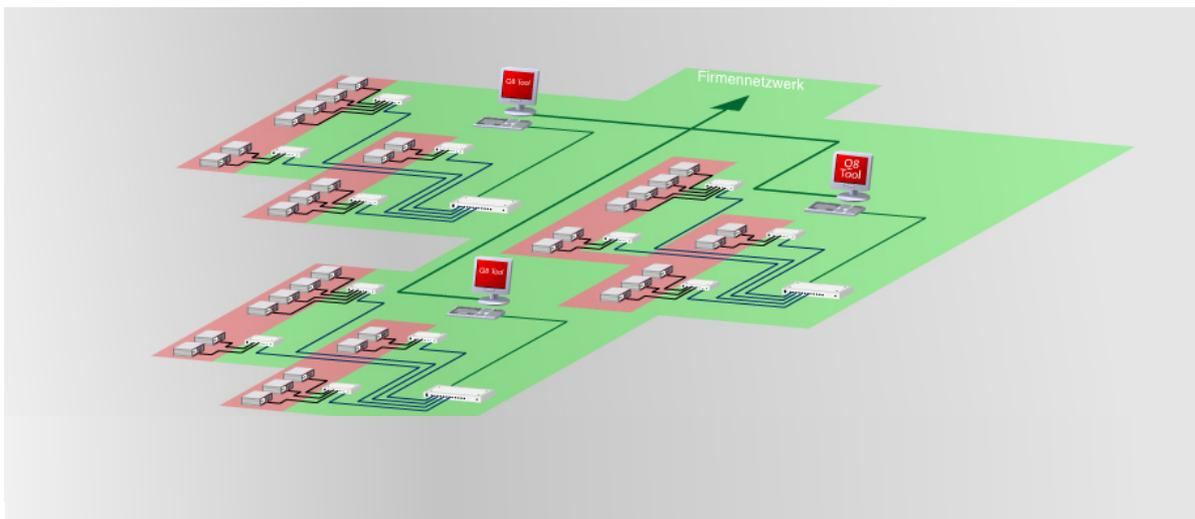
Networking with the Q8Tool software and further processing of the weld data with the help of the DCOM interface in the corporate network.
