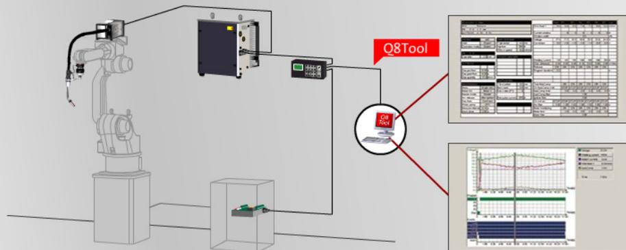
The cost optimized model is integrated into the power source. All other weld controller can be flexibly placed within the weld cell – for a perfect operationability.
